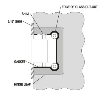
Check your walls with a straight edge. If the mounting is irregular the hinge may not function properly.
