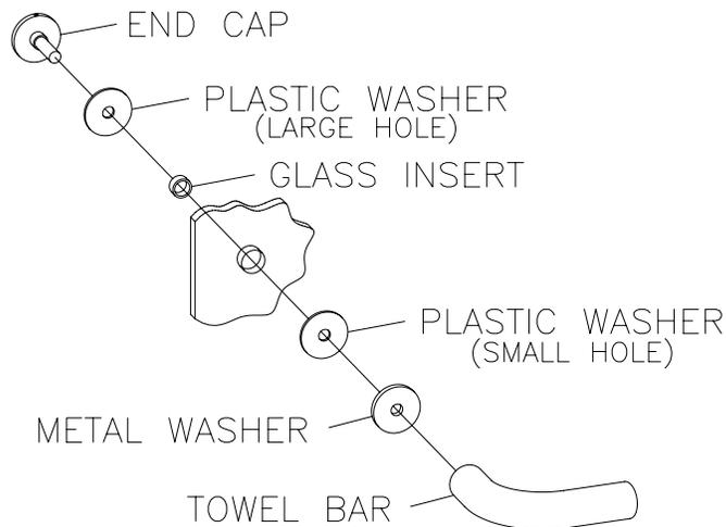
**11** Insert the wrench [S] into the small hole on the edge of an end cap [N] and rotate in a clockwise direction until tight. Repeat for all remaining end caps.
