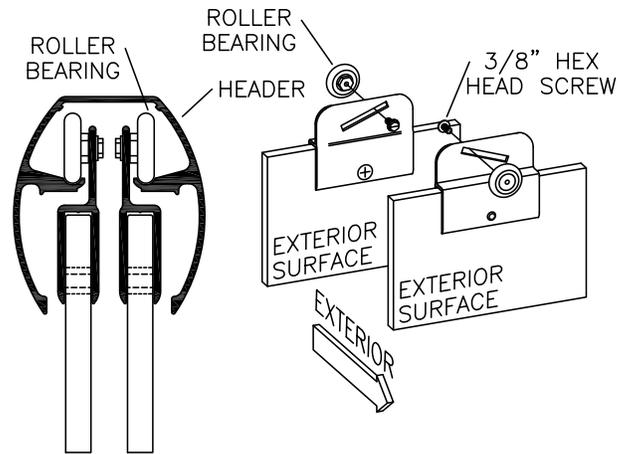
**8** Before installing the door panels, the proper orientation should be determined. For maximum water-proofing, the interior panel should always be positioned closest to the shower head, as shown in this illustration.
