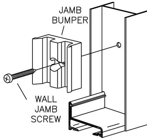
**5** This bath enclosure is equipped with safety tee-lock wall jambs. When installed properly the header is permanently locked to the wall jambs and cannot be accidentally dislodged.
