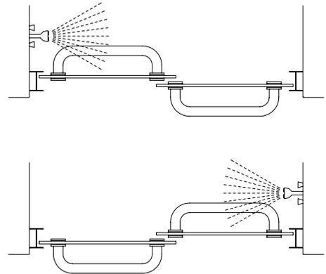
**9** Lift the interior door panel [H] (exterior surface closest to fin) into position with the roller bearings [K] engaging the roller slot in the header [F]. If the door panel is not parallel to the wall jambs, remove and adjust the roller bearings up or down to compensate. Repeat for the exterior door panel (exterior surface away from the fin).
