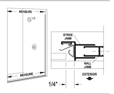
Inside the shower enclosure, drill two 1/8" holes thru the strike jamb [G] and into the wall jamb [C] 3/8" to 3/4" from the wall and approximately 1" vertically from each end of the strike jamb. Drill a third hole centered between the first two, then enlarge the three outer holes with a 3/16" drill for clearance on the self-tapping screws. Attach the strike jamb permanently with three  $\#6 \times 3/8"$ pan head screws [F].
