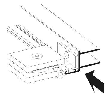
4 Lay the door glass [**B**] on a flat work surface and position the hinges [**Q**] by sliding them until they are lined up with the holes in the door glass. Remove the hinge plate and bushing. Position the door on the hinges and insert the plastic hinge bushing into the hole. Place the hinge plate on the glass, insert the hinge plate attachment screw and only tighten the screw enough to secure the hinge plate temporarily.
