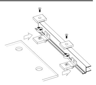
**5** Move the door panel [**B**] with hinges attached relative to the hinge jamb [**H**] until the top and bottom edges of the door glass are each 9/16" from the ends of the jamb. Mark the hinge mounting hole locations on the jamb. Detach the glass from the hinges by removing the hinge plate. Slide the hinges to the side and drill a 9/64" dia. hole at each location. Cut the seal vinyl to length to fit between the hinges and at each end of the hinge jamb. Slide the vinyl into the jamb as shown.
