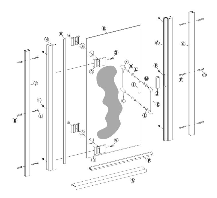
The Alumax 300D Continous Hinge Shower Door is completely reversible and may be installed hinge-left or hinge-right. Refer to the illustration to determine the correct position for your installation. For maximum waterproofing, the hinge jamb should always be opposite the shower head. These instructions depict a hinge-left installation.
