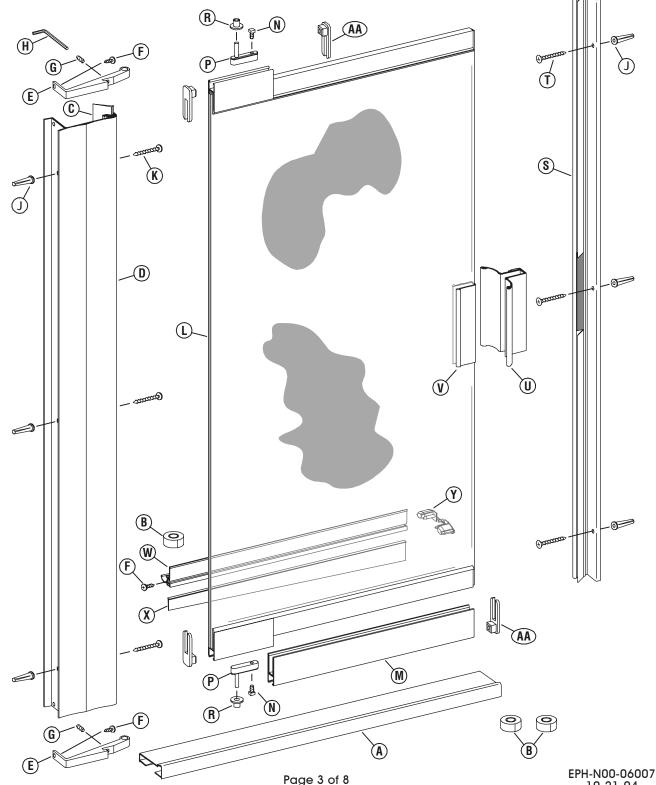
The ALUMAX 338 Frameless Pivot Shower Door is completely reversible and may be installed pivot-right or pivot-left. Refer to the illustration to determine the correct position for your installation. For maximum waterproofing, the pivot jamb should always be opposite the shower head. These instructions depict a pivot-left installation.
