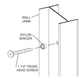
This bath enclosure is equipped with safety teelock wall jambs. When installed properly, the header is permanently locked to the wall jambs and cannot be accidentally dislodged.
