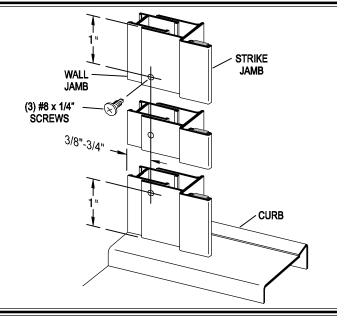
6 Slide the door panel [E] over the other wall jamb [B] until the door panel and the strike jamb [F] can meet. With the door closed and the latch magnets engaged, the proper door panel to strike jamb clearance is 1/8" (see illustration). Mark the hinge jamb's location on the wall jamb with a pencil.
