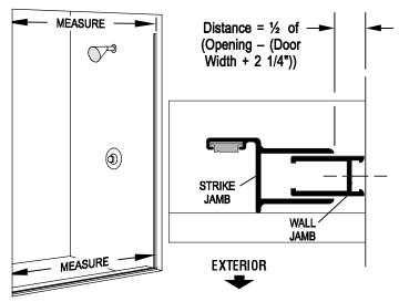
**5** Inside the shower enclosure, drill two 1/8" holes thru the strike jamb [**F**] and into the wall jamb [**B**] 3/8" to 3/4" from the wall and approximately 1" vertically from each end of the strike jamb. Drill a third hole centered between the first two, then enlarge the three outer holes with a 3/16" drill for clearance on the self-tapping screws. Attach the strike jamb permanently with three #8x 1/4" truss head screws [**G**].
