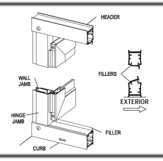
Pull the bottom end of the hinge jamb [J] tight to the curb filler [N] and plumb the jamb. Drill two 1/8" holes thru the hinge jamb and into the wall jamb 3/8" to 3/4" from the wall and approximately 1/4" vertically from the ends of the jamb. Drill a third hole centered between the first two and enlarge the outer holes with a 3/16" drill for clearance on the self-tapping screws. Attach the door panel permanently with three #8 x 1/4" truss head screws [L].
