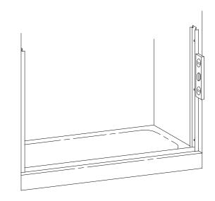
Before replacing the tub track [A], force a small downward bow into the extrusion. This will ensure the tub track [A] fits tight to the tub. Run 2 beads of caulk inside the penciled marks on the tub rim. Place the tub track [A] in the exact position marked in step #2 and seat it firmly in the caulking.
