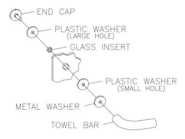
Insert the wrench [T] into the small hole on the edge of an end cap [I] and rotate in a clockwise direction until tight. Repeat for all remaining end caps.
