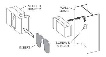
To install the optional bottom bumper [**U**], remove the bottom wall jamb screw closest to the shower head. Insert the screw through the hole in the center of the bottom jamb bumper and replace it in the wall jamb, with the leg pointing inside of the enclosure. Re-tighten the screw.
