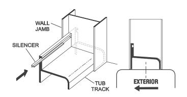
Use a level to plumb both wall jambs [B], then mark the pre-drilled hole locations on the wall. Lightly mark along both sides of the tub track [A] with a pencil, then remove all parts.
