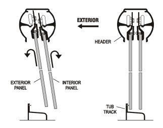
Locate the nylon bottom guide [**O**] in the middle of the tub track [**A**] with the glass panels in the position shown. With a 7/64" bit, drill two holes into the V-groove through the mounting holes in the guide. Install the bottom guide with two #6 x 3/8" pan head screws [**P**] thru the drilled holes as shown.
