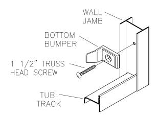
Neatly caulk each end of the tub track [A] where it meets the wall jambs [B] and the interior edge of the wall jambs as shown. Run a bead of caulking along the interior edge of the tub track.
