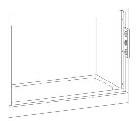
Before replacing the tub track [A], force a slight downward bow in the extrusion. This will ensure the track fits tight to the tub. Run two beads of caulk inside the penciled marks on the tub rim. Place the tub track in the exact position marked in Step #2 and seat it firmly in the caulking.
