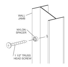
This bath enclosure is equipped with safety teelock wall jambs. When installed properly, the header is permanently locked to the wall jambs and cannot be accidentally dislodged.
