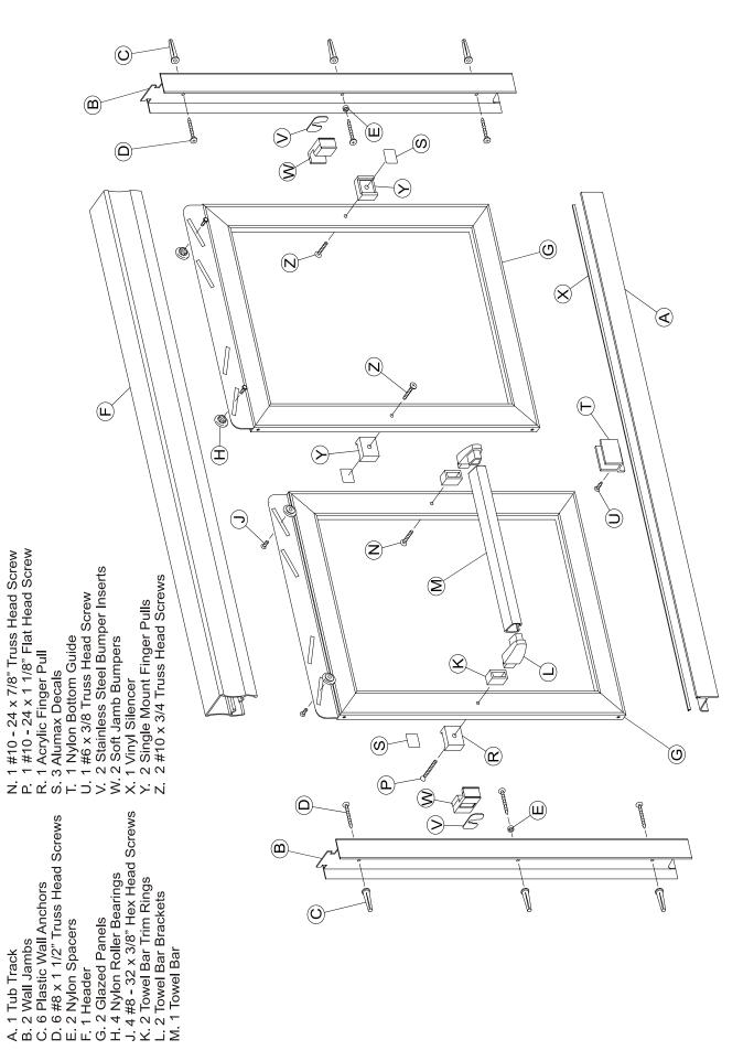
Measure the wall-to-wall opening at the center of the tub rim. Cut the tub track [A] 1/16" short of this dimension. An inexpensive miter box (available at your local hardware store) will help you get clean square cuts.
