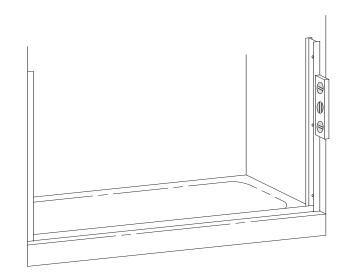
Before replacing the tub track [A], force a slight downward bow in the extrusion. This will ensure the track fits tight to the tub. Run two beads of caulk inside the penciled marks on the tub rim. Place the tub track in the exact position marked in Step #2 and seat it firmly in the caulking.
