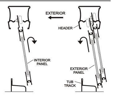
Before finishing the installation it is necessary to determine the proper closed position of the doors. For maximum water-proofing, position the interior panel closest to the shower head, as shown in the detail.
