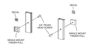
Attach a towel bar assembly (with the open slot in the bar downward) to the exterior panel with a #10-24 x 7/8" truss head screw [N] thru the inner rail. Insert a #10-24 x 1 1/8" flat head screw [P] thru an acrylic finger pull [R], thru the outer rail and into the outer towel bar bracket. Peel the backing from a ALUMAX decal [S] press it into the recess in the acrylic finger pull.
