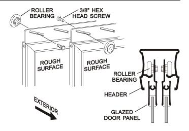
Lift the interior panel (with the rough surface closest to the top fin) into position with the rollers engaging the roller slot in the header **[F]**.
