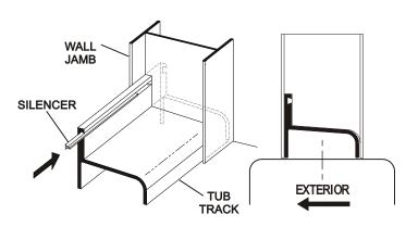
Use a level to plumb both wall jambs [B], then mark the pre-drilled hole locations on the wall. Lightly mark along both sides of the tub track [A] with a pencil, then remove all parts.
