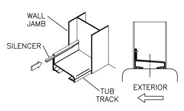
Use a level to plumb both wall jambs [**B**], then mark the pre-drilled hole locations on the wall. Lightly mark both sides of the tub track [**A**] with a pencil, and then remove all the parts.
