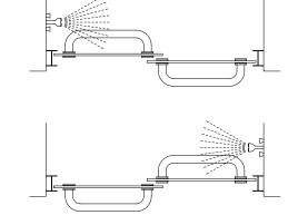
**9** Lift the interior door panel [H] (exterior surface closest to fin) into position with the roller bearings [K] engaging the roller slot in the header [F].
