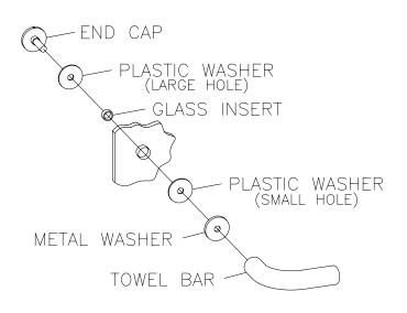
Insert the wrench [S] into the small hole on the edge of an end cap [N] and rotate in a clockwise direction until tight. Repeat for all remaining end caps.
