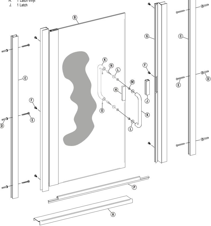
The Alumax 300cv Continous Hinge Shower Door is completely reversible and may be installed hinge-left or hinge-right. Refer to the illustration to determine the correct position for your installation. For maximum waterproofing, the hinge jamb should always be opposite the shower head. These instructions depict a hinge-left installation.
