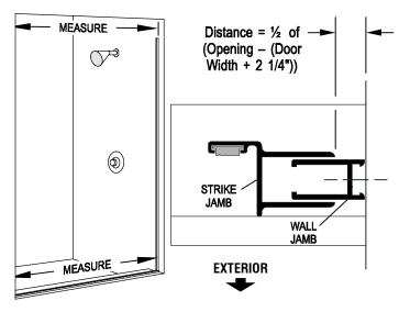
Inside the shower enclosure, drill two 1/8" holes thru the strike jamb [G] and into the wall jamb [C] 3/8" to 3/4" from the wall and approximately 1" vertically from each end of the strike jamb. Drill a third hole centered between the first two, then enlarge the three outer holes with a 3/16" drill for clearance on the self-tapping screws. Attach the strike jamb permanently with three #6 x 3/8" pan head screws [F].
