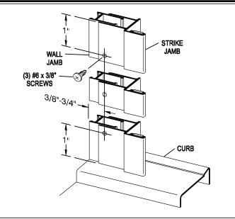
Slide the hinge jamb of the door panel assembly [B] over the mounted wall jamb [C] so the door will open outward.
