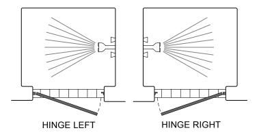
NOTE: The 300cv unit may be installed without using the sloped curb [A] provided. Its use is definitely recommended for positive water control on shower sills with little or no slope.
