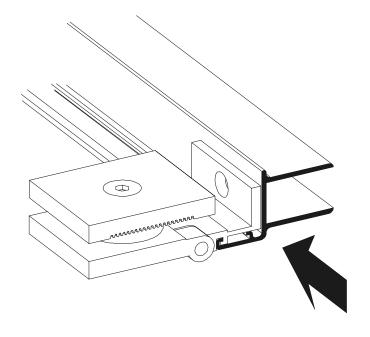
Lay the door glass [**B**] on a flat work surface and position the hinges [**Q**] by sliding them until they are lined up with the holes in the door glass. Remove the hinge plate and bushing. Position the door on the hinges and insert the plastic hinge bushing into the hole. Place the hinge plate on the glass, insert the hinge plate attachment screw and only tighten the screw enough to secure the hinge plate temporarily.
