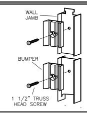
This bath enclosure is equipped with safety teelock wall jambs. When installed properly, the header is permanently locked to the wall jambs and cannot be accidentally dislodged.
