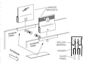
**CAUTION** – Do not over tighten the brackets and cause the end to clamp down on patterned glass. Do NOT use a screw gun. This can cause the glass panel to shatter.
