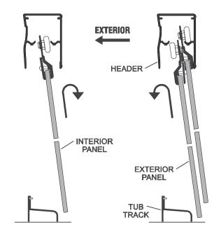
Locate the nylon bottom guide [**S**] in the middle of the tub track [**A**] with the glass panels in the position shown. With a 7/64" bit, drill two holes into the V-groove through the mounting holes in the guide. Install the bottom guide with two #6 x 3/8" pan head screws [**T**] thru the drilled holes as shown.
