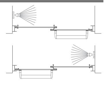
Lift the interior glass panel into position with the rollers engaging the groove in the header [F]. Repeat for the exterior panel. If panels are not parallel to their respective wall jambs, remove and adjust the rollers up or down in their slots to compensate.
