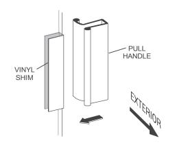
Before installing the door panels, the proper orientation should be determined. For maximum water-proofing, the interior panel should always be positioned closest to the shower head, as shown in this illustration.
