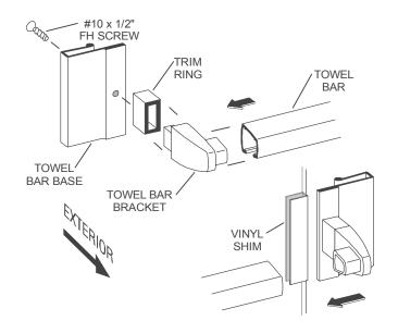
Press the two pull handles [R] and vinyl shims [P] into place on the interior glass panel at the same height as the towel bar bases [L] were mounted on the exterior panel.
