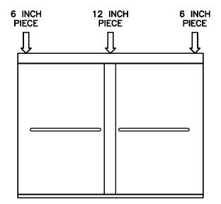
Measure the wall-to-wall opening along the center of the tub rim. Cut the tub track [**A**] 1/16" short of this dimension. An inexpensive miter box available at your hardware store will help you get clean square cuts.
