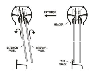
**11** Locate the nylon bottom guide [**O**] in the middle of the tub track [**A**] with the glass panels in the position shown. With a 7/64" bit, drill two holes into the V-groove through the mounting holes in the guide. Install the bottom guide with two #6 x 3/8" pan head screws [**P**] thru the drilled holes as shown.
