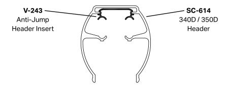
When installing the vinyl anti-jump into a new unit it is easiest to slide the vinyl into the end of the header before it is mounted to the frame. There are two 6 in pieces and a 12 inch piece. The 12 inch piece goes in the middle of the header with a 6 inch piece on either side of it. Install the header as described in the instruction sheet for your unit.
