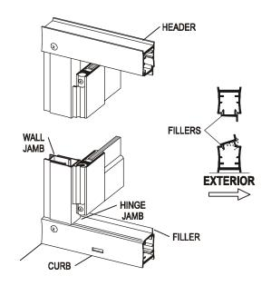
Pull the bottom end of the hinge jamb tight to the curb filler [\*C] and plumb the jamb. Drill two 1/8" holes thru the hinge jamb and into the wall jamb (or post) 3/8" to 3/4" from the wall and approximately 1/4" vertically from the ends of the jamb. Drill a third hole centered between the first two and enlarge the outer holes with a 3/16" drill for clearance on the self-tapping screws. Attach the hinge jamb/door panel permanently with three #8 x 1/4" truss head screws [\*D].
