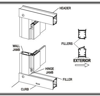
Pull the bottom end of the hinge jamb tight to the curb filler [\*C] and plumb the jamb. Drill two 1/8" holes thru the hinge jamb and into the wall jamb (or post) 3/8" to 3/4" from the wall and approximately 1/4" vertically from the ends of the jamb. Drill a third hole centered between the first two and enlarge the outer holes with a 3/16" drill for clearance on the self-tapping screws. Attach the hinge jamb/door panel permanently with three #8 x 1/4" truss head screws [\*D].
