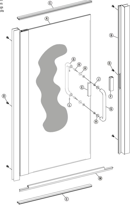
Press the hinge jamb/door panel assembly [\*A] and strike jamb [\*B] (with magnetic strip) over the wall jamb and/or framing posts. Refer to Step #1 of the STIKSTALL instruction sheet for the proper handing of the door.
