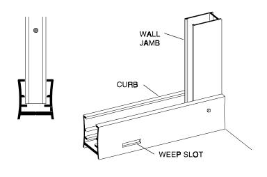
Wipe the shower walls and sill, the curb [A] and the wall jambs [B] with a clean, dry cloth to remove any dust or debris. Apply a 1/4" bead of caulk along the inside of both of the pencil lines marked in Step #2. Carefully replace the curb in the exact position marked. Caulk the inside of the curb ends where they meet the wall.
