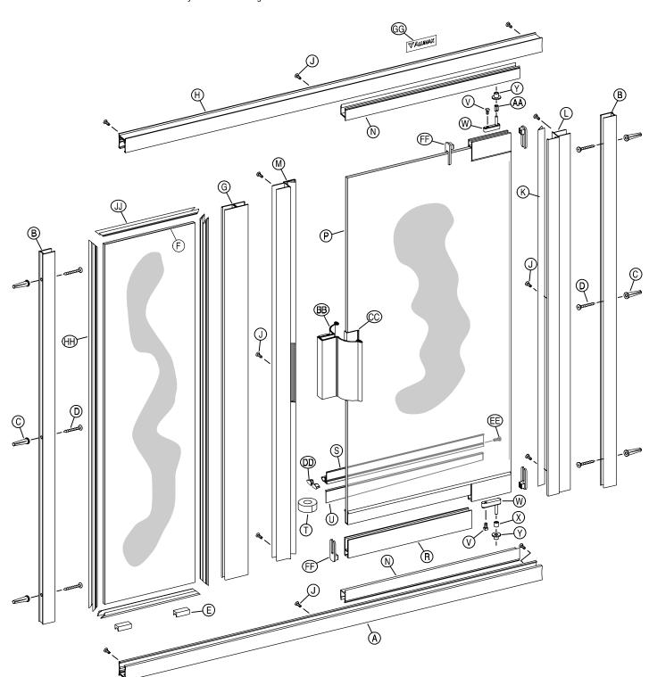
The Alumax 391 StikStall Shower Enclosure is completely reversible and may be installed pivot-left or pivot-right. The door may pivot from the wall or from the center post. For maximum waterproofing, the pivot jamb should always be opposite the shower head. Using the illustration, determine the correct position for the door in your particular StikStall installation. This instruction sheet depicts a pivot-right installation.
