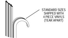
Cut four pieces of the smaller vinyl [JJ] 1" longer than the vertical opening (to prevent gapping from shrinkage) and trim the ends on a 45° angle. Using the masking tape guides, center the glass panel [J] in the frame. Cut four short (1" - 2") pieces of the small vinyl and press into the jamb and post on each side to hold the glass temporarily.
