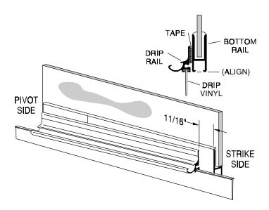
Adjust the drip vinyl [V] by sliding it left or right until it just touches the curb. Trim the vinyl (flush with the pivot end and notch 1/2" longer than the drip rail as shown on the strike end). Secure it with one #6 x 3/8" truss head screw [FF] in the pivot end of the drip rail [T].
