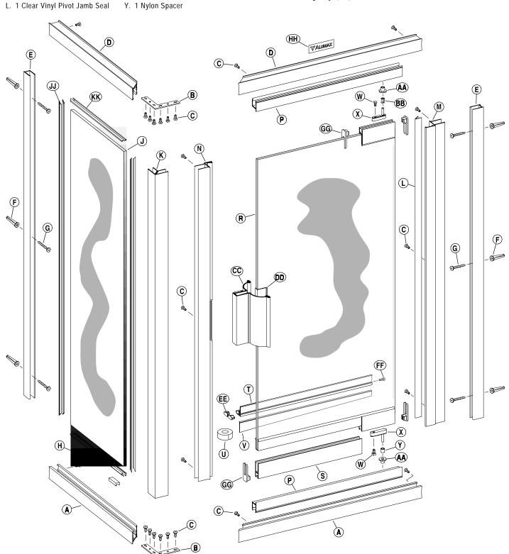
The Alumax 392 StikStall Shower Enclosure is completely reversible and may be installed pivot-left or pivot-right. The door may pivot from the wall or from the center post. Using the illustration, determine the correct position for the door in your particular StikStall installation. This instruction sheet depicts a pivot-right installation.
