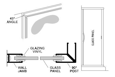
Cut four pieces of the larger vinyl [KK] 1/2" longer than the horizontal opening and trim the ends on a 45° angle. Install the top exterior vinyl starting at both ends and working toward the middle. Be careful not to stretch the vinyl.
