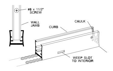
Place two plastic setting blocks [H] into the curb assembly [A] to support the fixed glass panel [J]. Position the blocks 3" from each corner of the glass panel. Remove any protective strips from the glass panel and set into place on the setting blocks and approximately 1/2" into the wall jamb [E]. A strip of masking tape 1/2" from each vertical edge of the glass will aid alignment.
