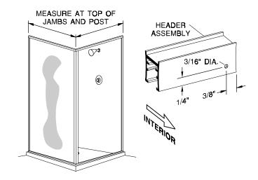
Press the header assembly [**D**] over the wall jambs [**E**] and the 90° post [**K**]. Check the post for plumb. Adjust as required by varying the overlap of the header over the wall jambs. In some cases, you may need to trim the ends of the header where it meets the wall. The minimum horizontal dimension for the door opening is the door panel width (see the graphic in Step **#9**) plus 1/2", maximum is the door panel width plus 1 3/4".
