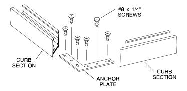
Measure the opening at the bottom of the shower stall and trim the ends of the curb assembly [A] (with weep slots) to fit the shower sill. The curb should sit near the centerline of the sill. If required, use a file to round the lower ends of the curb assembly to fit the shower sill properly.
