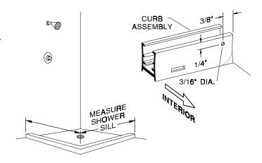
Place the two wall jambs [E] into the ends of the curb assembly [A]. Masking tape may be used to hold the curb in place during this operation. Plumb the jambs and mark the hole locations on the wall. Remove all parts and drill the walls for mounting hardware.
