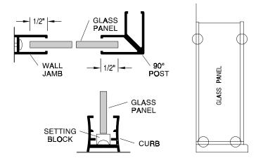
Hold the 90° post [K] plumb and carefully measure horizontally from the top of each wall jamb [E] to the outside edge of the post. Add 3/16" to each measurement to find the corresponding dimension on the header assembly [D] (from the outside mitered edge to the squared ends) and trim the header assembly to fit.
