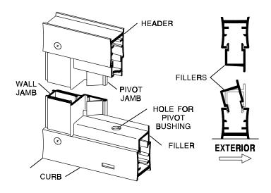
Pull the bottom end of the pivot jamb [M] tight to the curb filler [P] and plumb the jamb. Drill two 1/8" holes thru the pivot jamb and into the wall jamb [E] 3/8" to 3/4" from the wall and approx. 1/4" from the ends of the jamb. Drill a third hole centered between the first two, then enlarge the three outer holes with a 3/16" drill for clearance on the self-tapping screws. Attach the pivot jamb permanently with three #8 x 1/4" truss head screws [C].
