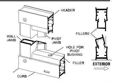
Pull the bottom end of the pivot jamb [N] tight to the curb filler [R] and plumb the jamb. Drill two 1/8" holes thru the pivot jamb and into the wall jamb [E] 3/8" to 3/4" from the wall and approximately 1/4" from the ends of the jamb. Drill a third hole centered between the first two, then enlarge the three outer holes with a 3/16" drill for clearance on the self-tapping screws. Attach the pivot jamb permanently with three #8 x 1/4" truss head screws [C].
