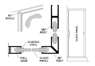
Cut eight pieces of the larger vinyl [LL] 1/2" longer than the horizontal opening and trim the ends on a 45° angle. Install the top exterior vinyl starting at both ends and working toward the
