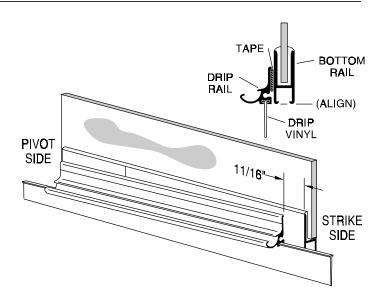
Adjust the drip vinyl [W] by sliding it left or right until it just touches the curb. Trim the vinyl (flush with the pivot end and notch 1/2" longer than the drip rail as shown on the strike end). Secure it with one #6 x 3/8" truss head screw [GG] in the pivot end of the drip rail [U].
