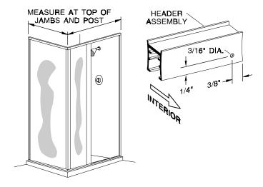
Press the header assembly [**D**] over the wall jambs [**E**], 90° post [**K**] and 180° post [**L**]. Check the posts for plumb. Adjust as required by varying the overlap of the header over the wall jambs. You may need to trim the ends of the header where it meets the wall. The minimum horizontal dimension for the door opening is the door panel width (see the graphic in Step **#9**) plus 1/2", maximum is the door panel width plus 1 3/4".
