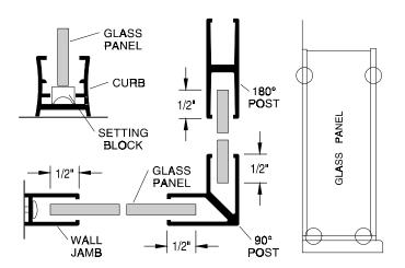
Hold the 90° post [K] plumb and carefully measure horizontally from the top of each wall jamb [E] to the outside edge of the post. Add 3/16" to each measurement to find the corresponding dimension on the header assembly [D] (from the outside mitered edge to the squared ends) and trim the header assembly to fit.
