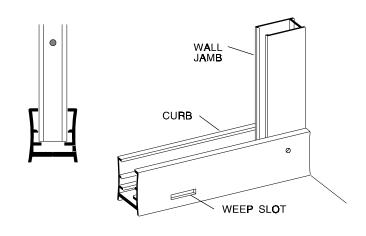
Wipe the shower walls and sill, curb assembly [A], and wall jambs [E] with a clean, dry cloth to remove any dust or debris. Apply a 1/4" bead of caulk along the inside of both of the pencil lines marked in Step #3. Carefully replace the curb in the exact position marked. Caulk the inside of the curb ends where they meet the wall. Caulk generously around the anchor plate [B], screws [C], and the inside of the mitered joint.
