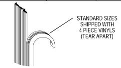
Cut eight pieces of the smaller vinyl [KK] 1" longer than the vertical opening (to prevent gapping from shrinkage) and trim the ends on a 45° angle. Using the masking tape guides, center the first glass panel [J] in the frame. Cut four short (1" - 2") pieces of the small vinyl and press into the jamb and post on each side to hold the glass temporarily.
