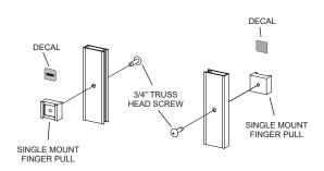
Attach a towel bar assembly (with the open slot in the bar downward) to the exterior panel with a #10-24 x 7/8" truss head screw **[N]** thru the inner rail. Insert a #10-24 x 1 1/8" flat head screw **[P]** thru an acrylic finger pull **[R]**, thru the outer rail and into the outer towel bar bracket. Peel the backing from a ALUMAX decal **[S]** press it into the recess in the acrylic finger pull.
