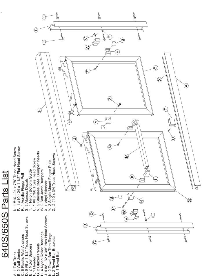
Measure the wall-to-wall opening at the center of the tub rim. Cut the tub track **[A]** 1/16" short of this dimension. An inexpensive miter box (available at your local hardware store) will help you get clean square cuts.
