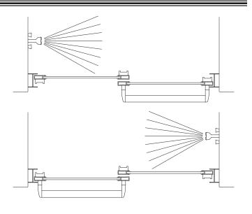
9 Slide the two towel bar trim rings **[K]** over the clear acrylic towel bar brackets **[L]** and press the brackets into the ends of the towel bar **[M]**.
