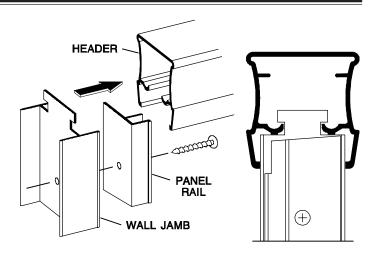
Cut the inline panel vinyls [H] to the length of the long edges of the inline glass panel [J] and press them onto the edges of the panel. Stand the panel upright on the tub track [A] and press it into the mounted inline panel rail [G]. Press the second panel rail over the other edge of the glass panel and vinyl with the bottom of the panel rail flush against the tub track.
