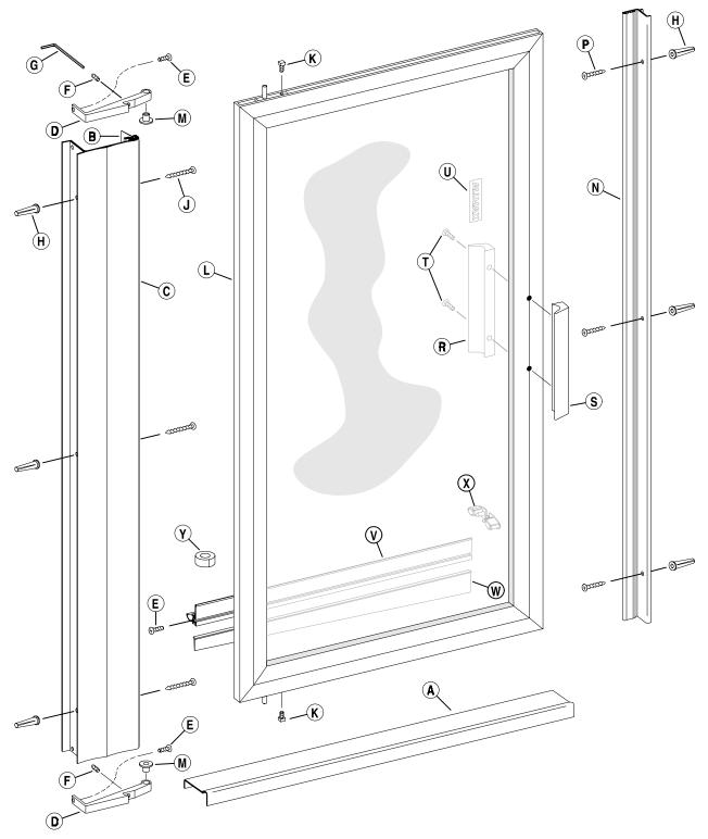
The ALUMAX 738 Pivot Shower Door is completely reversible and may be installed pivotright or pivot-left. Using the diagram, determine the correct position for your installation. For maximum waterproofing, the pivot jamb should always be opposite the shower head. These instructions depict a pivot-left installation.
