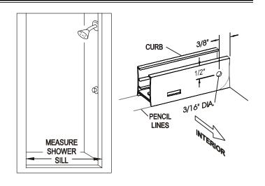
Place the two wall jambs [C] into the ends of the curb [A]. Masking tape may be used to hold the curb in place during this operation. Plumb the jambs and mark the hole locations on the wall. Remove all parts and drill the walls for mounting hardware.
