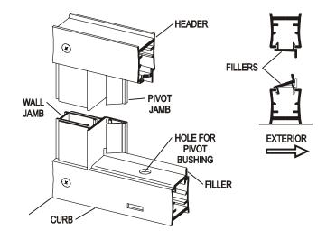
Pull the bottom end of the pivot jamb [N] tight to the curb filler [R] and plumb the jamb vertically. Drill two 1/8" holes thru the pivot jamb and into the wall jamb [C] 3/8" to 3/4" from the wall and approximately 1/4" vertically from the ends of the jamb. Drill a third hole centered between the first two and enlarge the outer holes with a 3/16" drill for clearance on the self-tapping screws. Attach the pivot jamb permanently with three #8 x 1/4" truss head screws [L].
