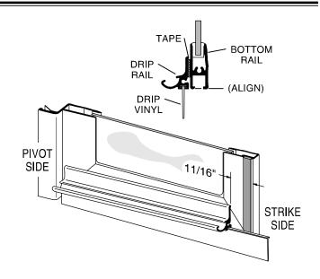
Adjust the drip vinyl [U] by sliding it left or right until it just touches the curb. Trim the vinyl (flush with the pivot end and notch 1/4" longer than the drip rail as shown on the strike end).
