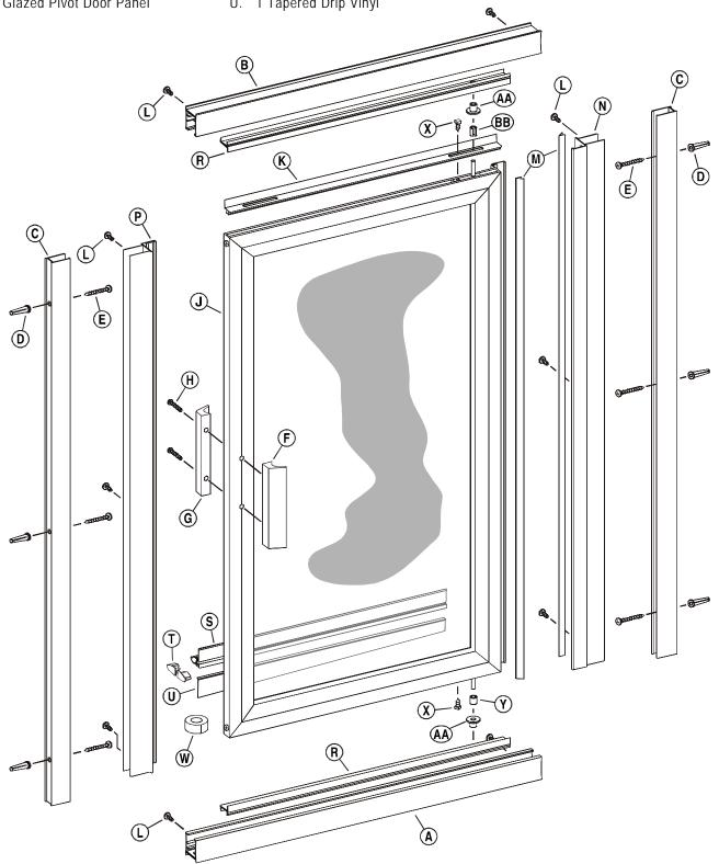
The Alumax 890 Steam Door is designed to be installed alone as shown in the exploded views or combined with a custom StikStall framework. They can be installed with an inline panel (091), a return panel (092), an inline and a return panel (093), or a neo-angle unit (094). Fixed glass panel sizes should be determined by formulas shown on Alumax detail sheets.
