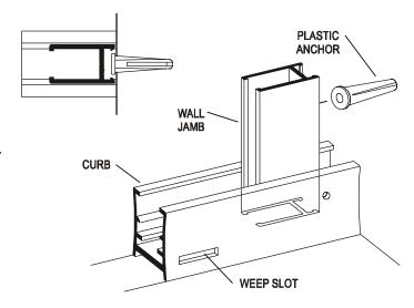
Wipe the shower walls and sill, curb [A] and wall jambs [C] with a clean, dry cloth to remove any dust or debris. Apply a 1/4" bead of caulk along the inside of both of the pencil lines marked in Step #2. Carefully replace the curb in the exact position marked. Caulk the inside of the curb ends where they meet the wall.
