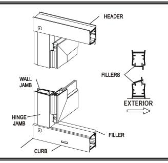
Pull the bottom end of the hinge jamb [J] tight to the curb filler [N] and plumb the jamb. Drill two 1/8" holes thru the hinge jamb and into the wall jamb 3/8" to 3/4" from the wall and approximately 1/4" vertically from the ends of the jamb. Drill a third hole centered between the first two and enlarge the outer holes with a 3/16" drill for clearance on the self-tapping screws. Attach the door panel permanently with three #8 x 1/4" truss head screws [L].
