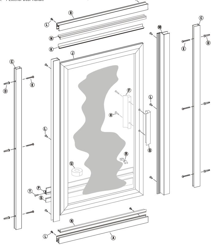
The Alumax 890 Continuous Hinge Steam Door is designed to be installed alone as shown in the exploded view or combined with a custom StikStall framework. It can be installed with an inline panel (091), a return panel (092), an inline and a return panel (093), or a neo-angle unit (094). Fixed glass panel sizes should be determined by formulas shown on Alumax detail sheets.
