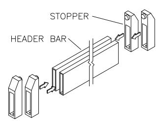
4 Set the header bar and stopper assembly into the wall mount bracket, from the top. Slide a Wall Mount Cover [G] into the wall mount bracket. Tighten the wall mount, and wall mount cover set screws [H] until the header bar is secure. This will prevent rattles in the header bar.
