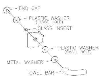
Insert the wrench (in the towel bar box) into the small hole on the edge of an end cap and rotate in a clockwise direction until tight. Repeat for all remaining end caps.
