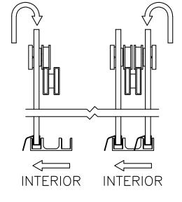
**10** For maximum water-proofing, the interior panel should always be positioned closest to the shower head, as shown in this illustration.
