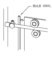
**12** Set the Stops – Move the door to the closed position. Slide the Stopper [BB] over until it touches the top roller on the strike side of the door. Tighten the Stopper Set Screw [CC] with the bumper in the up position. Move the door to the open position with the handle 1/4" - 1/2" from hitting the fixed panel. Slide the other stopper over until it just touches the top roller on the fixed side of the door. Tighten the Stopper Set Screw with the bumper in the up position.
