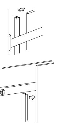
Set the Stops – Move the door to the closed position. Slide the Stopper [AA] over until it touches the roller on the strike side of the door. Tighten the Stopper Set Screw [BB]. Move the door to the open position with the handle 1/4" - 1/2" from hitting the fixed panel. Slide the other stopper over until it just touches the roller on the fixed side of the door. Tighten the Stopper Set Screw.
