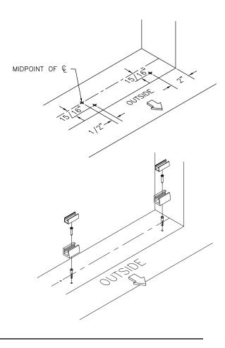
Center Guide – Make a mark on the centerline approximately 1 1/2" toward the door side. Place the Center Guide [L] on the new mark, centered on the mark. Mark the center of the attachment holes and, remove the Center Guide. Drill two 5/16" holes at the center guide attachment locations. Clean the area around the holes and put a little silicone into each hole. Press the Center Guide Anchors [M] into the holes. Mount the Center Guide with the Center Guide Screws [O].
