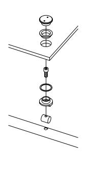
Fixed Panel Installation - Install the "peel-and-stick" Wall Seal [I I] on the wall side edge of the Fixed Panel. Orient it with the open end to the inside of the enclosure. Lift the Fixed Panel and set it in the Glass Clips with the edge as tight to the wall as possible. Loosen the Set Screws in the wall mount sleeves and slide them over the Wall Mount Blocks. Snug the Set Screws into the block (**DO NOT TIGHTEN**).
