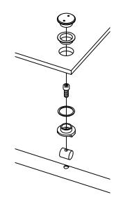
**9** Fixed Panel Installation - Install the "peel-and-stick" Wall Seal [I I] on the wall side edge of the Fixed Panel. Orient it with the open end to the inside of the enclosure. Lift the Fixed Panel and set it in the Glass Clips with the edge as tight to the wall as possible. Loosen the Set Screws in the wall mount sleeves and slide them over the Wall Mount Blocks. Snug the Set Screws into the block (**DO NOT TIGHTEN**).
