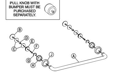
Hold the acrylic towel bar assembly against the threaded handle bases and screw the outer handle rings onto the bases. Do not overtighten or use tools that might damage the finish.
