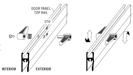
Close the door and rotate the exterior handle 90° downward causing the interior handle to rotate 90° upward and contacting the inside header surface. The interior handle will put pressure on the inside of the header keeping the door closed for transportation.
